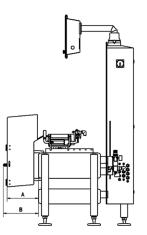
The scale drawing shows Flexus<sup>®</sup> with a collection container (optional), which is made from plastic or stainless steel – both versions have different dimensions.
